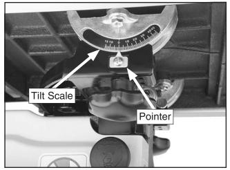
Figure 38. Location of the table tilt scale.
